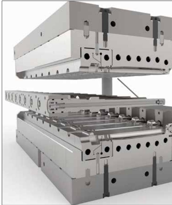
**Developed over time, the Liberty injection blow molding tooling system from R&D/Leverage features a variety of innovations to compensate for thermal expansion, improve alignment and simplify maintenance.**
